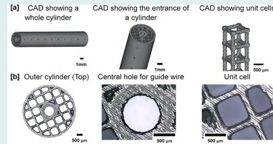
**Figure 2.** Design of the 3D printed porous cylinder using computer-aided design (CAD) and optic micrographs of its interior.<sup>4</sup>
