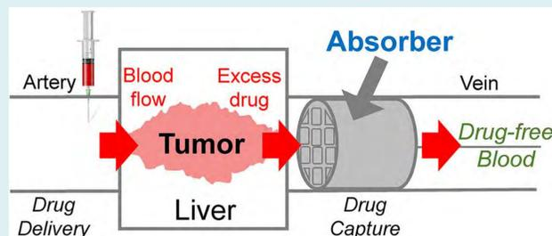
**Figure 1.** The proposed approach of 3D printing an absorber for drug capture.<sup>4</sup>
