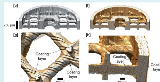
**Figure 3.** Magnified views of the uncoated (gray) and coated (orange) absorbers at different locations.<sup>4</sup>
